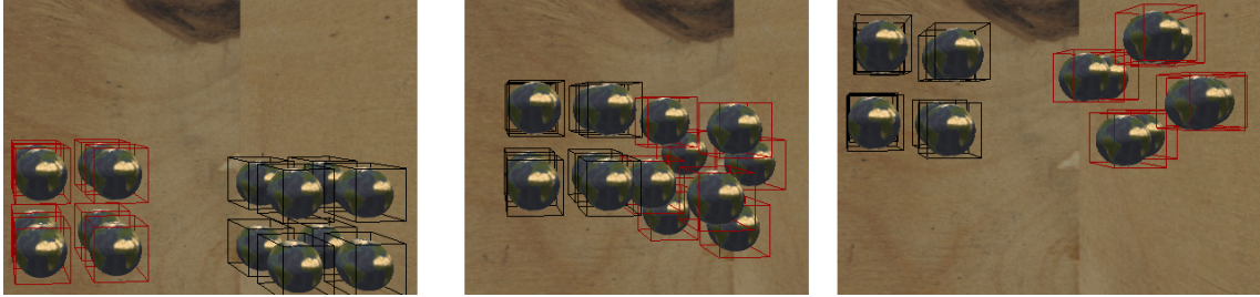
Figure 2.3: An example of collision detection working only on the particles of the objects. The particles are large and bunched closely together so that when the two objects meet, they do not intersect.
